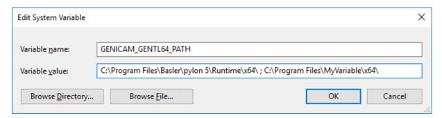
If there is no variable like that you need to create one using appropriate name (GENICAM\_GENTL64\_PATH / GENICAM\_GENTL32\_PATH) and the path to the folder that was created earlier.
