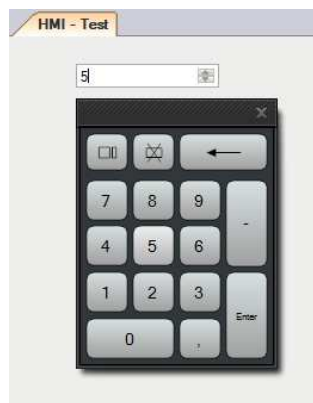
The example of using VirtualKeyboard for entering data on HMI panel into NumericUpDown control.
