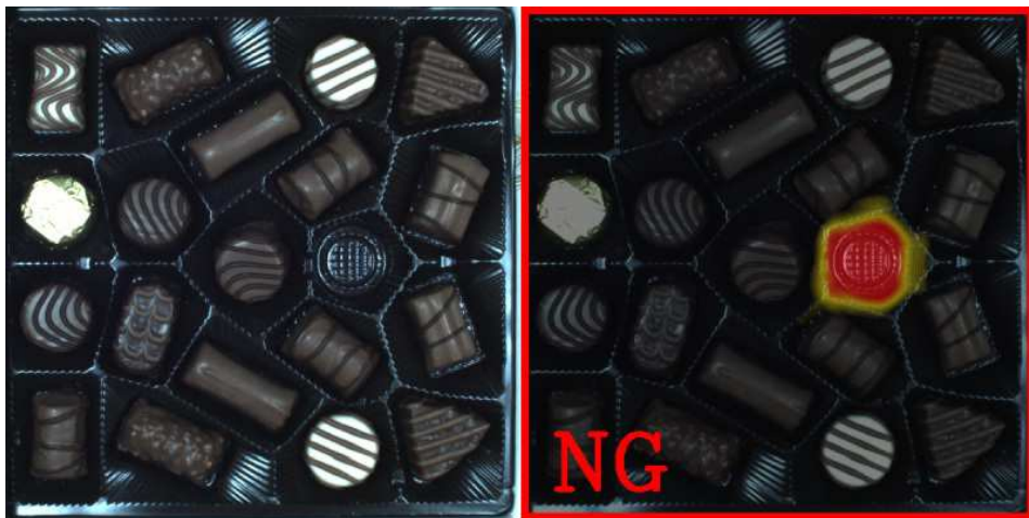
An example of missing part detection using DeepLearning_DetectAnomalies2 tool. Left: The original image with a missing element. Right: The classification result with a heatmap of defects overlay.
