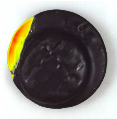
An example of cookie shape defects detection using the Global processing of the DeepLearning_DetectAnomalies1 filter.
